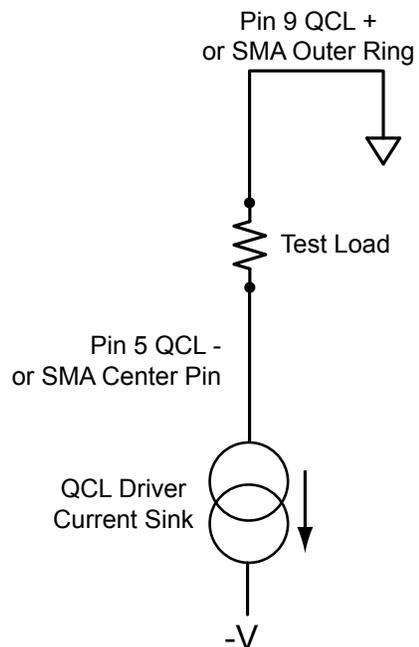
**Figure 14. Test Load Polarity Diagram**
