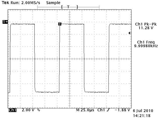
Figure 23. 10 kHz Output Plot
