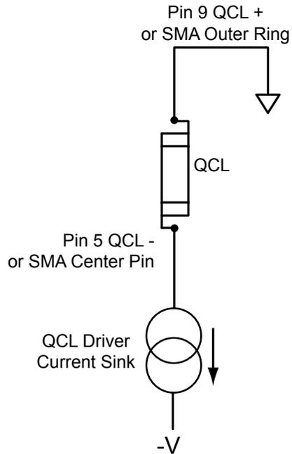
**Figure 4. QCL Polarity Diagram**
