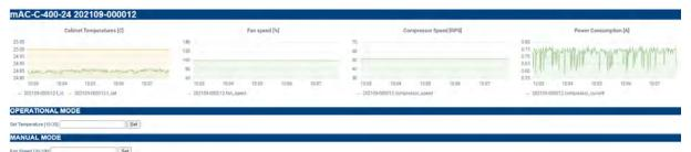
The mAC-C-400-24 is "IoT ready" – an integrated Ethernet interface allows remote access to system parameters as well as remote control of the cooling system via a web browser.
