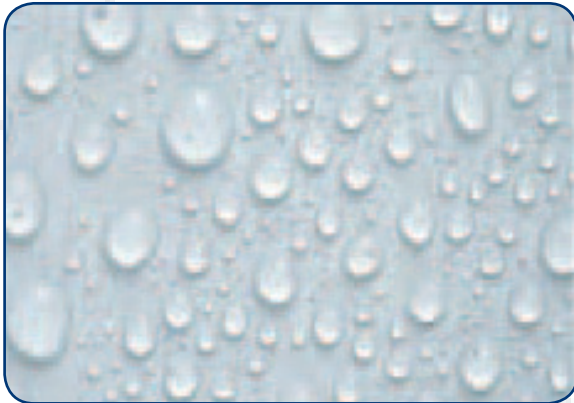
Ordinary Coating: Water Film and Large Droplets
