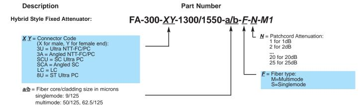
Note: Hybrid style attenuators with angled finishes must have matching style connectors one each end (i.e. Angled NTT-FC/PC to Angled NTT-FC/PC, not Angled NTT-FC/PC to Angled SC or Angled NTT-FC/PC to Ultra NTT-FC/PC
