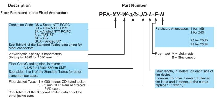
Note: Add -(HP) to the end of the part number for attenuated high power patchcord style.
