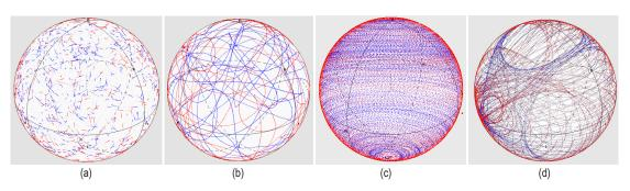
Figure 1. Poincaré sphere SOP traces for four different scrambling methods: (a) Discrete, (b) Typical Rayleigh or Triangle trace, (c) Tornado (fixed axis), and (d) Tornado (rotating axis).
