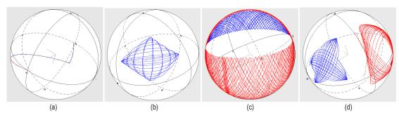
Figure 3. (a) Manual adjustment of SOP from H to V state. (b-d) SOP patterns generated in polarization modulation mode using different combinations of waveforms on different channels of the polarization controller.
