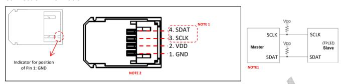
NOTE 1: The SCLK and SDAT pins are open collector. Apply appropriate pull up resistors on the SMBus master device.
