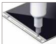
Conductive Ag paste dispensing on touch panels
