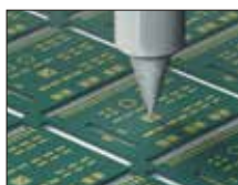
Ag paste dispensing for die bonding
