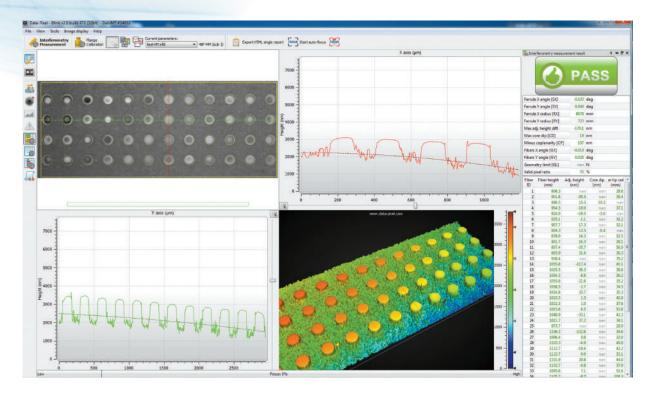
Blink is a software platform common to all Data-Pixel products. Dedicated plugins support the Interferometry range of products: 3D Scope-V2, Daffi SF, Daisi-V3, Daffi MT and Daisi MT FP.
