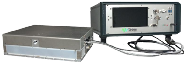
Picture of the prototype of the Mid-IR OPO compact source (on the left) and its controller (on the right)
