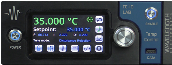
Figure 22. PID Coefficients automatically recalculated for Tune mode change
