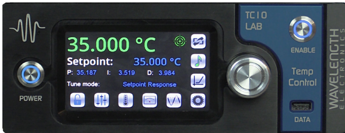
Figure 18. PID Coefficients automatically recalculated for setpoint change
