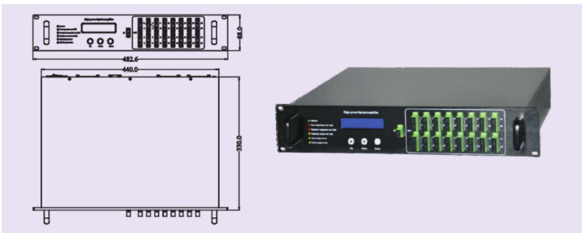
Mechanical Outline: 19-in 2U Rack (typical)
