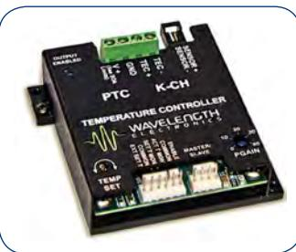
AMS Technologies offers a range of high-precision, ultra-stable temperature controllers for thermo-electric cooler modules. A very common application is the temperature control of laser diodes. Our controllers provide
