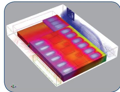
Thermal simulation with computational fluid dynamics (CFD) allows the engineer to dimension his system in great detail. Especially in complex systems life expectancy of electronic components, space, mass and cost may be optimized. The analysis of temperatures and air flows helps to take the right measures such as adjusting air flow, positioning of power components, dimensioning of heat sinks and fans and others. AMS Technologies has done more than 230 studies for customers since the year 2000.
