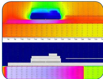
Safe operation at high ambient temperature required two peltier modules. Conventional high-performance heat sinks are not good in heat spreading and a high temperature difference creates a 300 W heat load on the hot side of a single peltier for a 60 W laser diode. The solution was to operate peltier modules in more efficient mode and distribute power on two modules.
