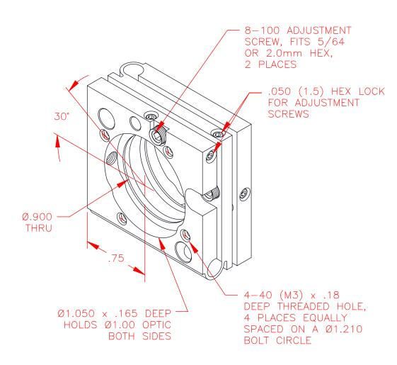
DIMENSIONS IN PARENTHESES REFLECT METRIC ASSEMBLY FEATURES
