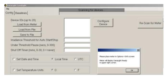
(note you can perform these steps in any order, If you initiate software first, when see a no devices connected error message, simply plug in the meter, turn it on, place in Data Ready Mode and then "Re-Scan for Meter" in the software.)
