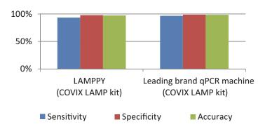
In a lab study done at Acibadem University using saliva samples taken from patients at the Acibadem Hospitals, LAMPPY was compared to a well-known conventional qPCR machine in performance and speed. The comparison study was carried out with a sample size of 262 using the COVIX LAMP-based kit on both instruments and then verified with the KrosQuanT SARS-COV-2 (2019 nCOV) Real Time PCR Diagnostic Kit on a leading brand conventional qPCR machine.
