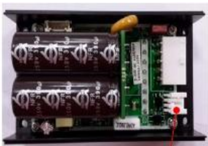
Outer LED source in Molex 53426-0310 #2 Pin
