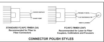
polarization maintaining capabilities compared to physical contact style couplers. However because of the air gap between the fiber and the lens, the backreflection level for the endface of the fiber is about -14dB. This can be reduced to -40dB to -60dB by slant polishing both fiber ends to deflect the backreflected signal.
