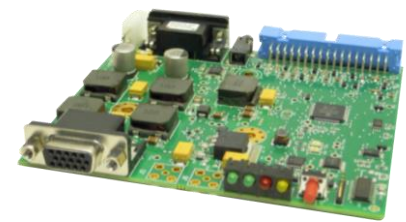
Board MLC-03A-BR1 or MLC-05A-BR1 for OEM lasers using 12V DC
