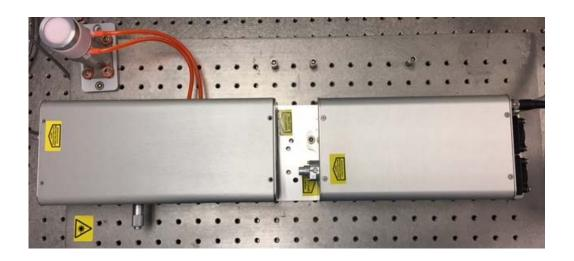
The position of the two heads, as factory tested, is marked by labels. Bolt down the SPOT and Dye laser heads to the plate using M6 bolts. (It will be necessary to take the lid off the dye laser to access the bolt holes). Align the edges of the heads to the edges of the plate. The heads could also be mounted directly to an optical table or breadboard with similar spacing.
