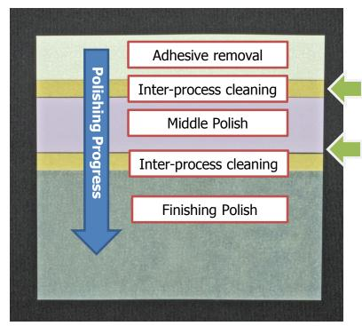
By placing a buff film between each of the polishing films, the polishing and inter-process cleaning are done at one time as a batch.
