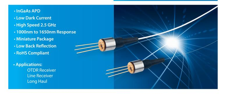
The LAPD 3050 is a 50um InGaAs APD housed in a hermetic 3 pin coaxial package. The APD is coupled to a singlemode fiber pigtail. The low noise, overload tolerant LAPD 3050 coax APD makes the devices ideal for OTDRs, line receivers and any other light level detection/ signal transmission application.
