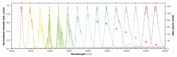
Representative instantaneous bandwidth as the OPO is tuned across its full range. Water absorption lines can be observed across the 5.5 – 7.5 µm range. Chromacity follows a policy of continuous improvement, therefore, specifications are subject to change without notice.
