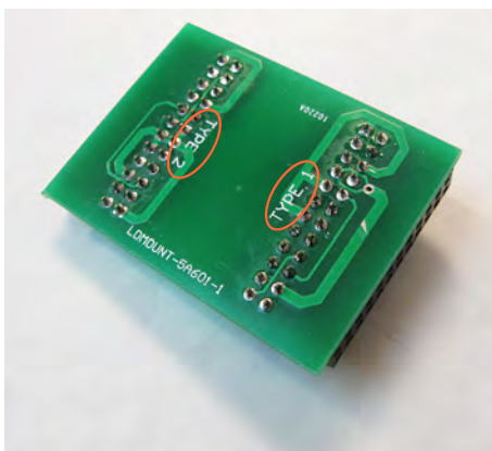
Figure 4. Pre-configured connection card. Allows operation of either a Type 1 or Type 2 laser.
