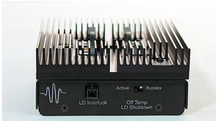
Figure 9. Interlock & Bypass side of the LDMOUNT. Interlock connection is on the left. Bypass switch is on the right.
