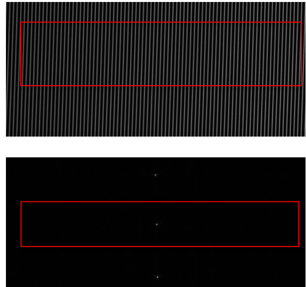
Figure 7: Typical CMOS sensor displays when the HyperFine spectrometer is illuminated with broadband light (upper), and a narrow-line-width monochromatic laser (lower). The full spectrum can be extracted by “unwrapping” the information in the regions marked with a box.
