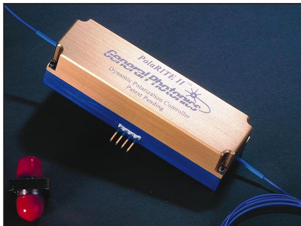
Figure 4. A fiber-squeezer-based dynamic polarization controller.
