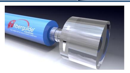
Fiberguide's end capped fiber optic assemblies allow the user to achieve higher coupled power into a fiber core by reducing the power density at the air/ silica interface, commonly the point of laser damage. End cap diameters and lengths are offered for select numerical apertures and fiber cores size, but can be easily customized for a variety of fiber types and specialized applications.
