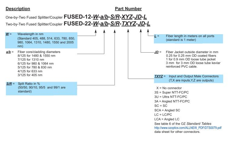
**Example:** The customer requires a singlemode two-by-two 50/50 coupler for 633nm (fiber core size is 4/125 for 633nm singlemode fiber). All ends are to be 0.5 meters long, cabled, and terminated with FC style connectors, Super PC finish. OZ Optics' part number: **FUSED-22-633-4/125-50/50-3S3S3S3-3-0.5**.
