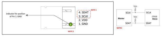
**NOTE 1**: The SCLK and SDAT pins are open collector. Apply appropriate pull up resistors (e.g. 4.7 kOhm) on the SMBus master device. **NOTE 2**: Module connector employed: CVILUX CI0104M1HR0-LF or JST S4B-PH; or equivalent.
