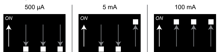
Figure 9. Proper PD RANGE DIP switch orientation for 500 \mu A, 5 mA, and 100 mA range.
