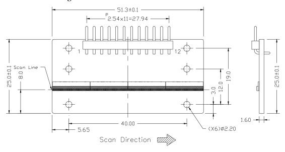
xxi Unit: Dimensions are in millimeters (mm).
