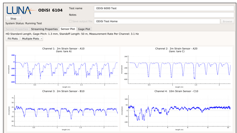
Multichannel sensor plot (strain/temperature versus length) in the ODiSI application software
