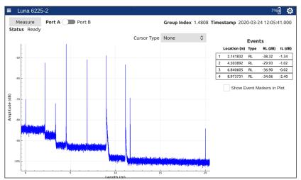
The OBR 6225 maps reflection versus length with high resolution, automatically detecting RL reflection events and IL sites that exceed user defined thresholds
