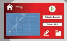
Intuitive software interface Integrated thermocouple moni tors curing block for precise temperature control 4 Independent timers to maximize small batch throughput
