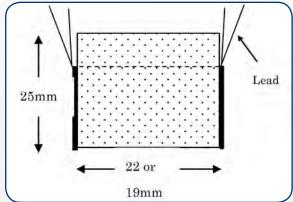
In order to focus the heating energy in this small volume and to minimize the losses to the environment, the actual heating element is enclosed in a very high heat resistant ceramic material. An approx. 1 mm wide gap in this material on one side makes the laterally open, tubular heating element accessible from the outside.
