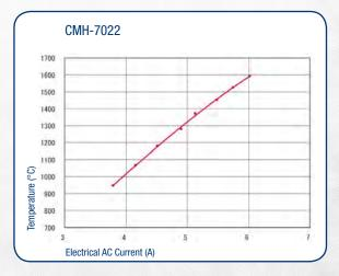
The conditions for this relationship between current and temperature may shift gradually during mid- to long-term operation. Therefore, temperature calibration using a 0.3 mm diameter, type B thermocouple is recommended once a month. This thermocouple has to be enclosed in a ceramic capillary to prevent damage caused by the high temperature.
