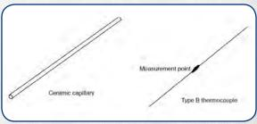
For calibration, put the thermocouple into the ceramic capillary and position the thermocouple joint (measuring point) to the center of the capillary to avoid damage and obtain the precise temperature. Then insert the capillary containing the thermocouple into the heater and measure the temperature with the help of a thermometer device suitable for thermocouples.
