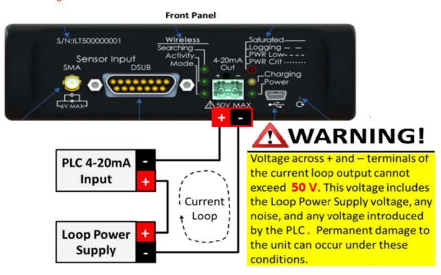
B. Connection: The 4-20mA current loop is connects as illustrated above. The Loop Power Supply provides the power for the current loop, and the ILT5000 controls the level of current that flows through the loop.
